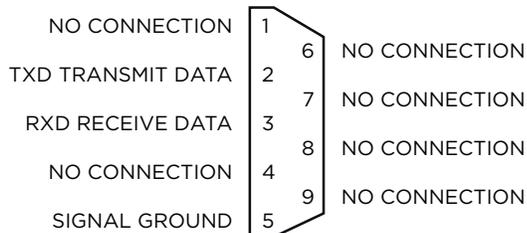
The OLS10K series is configured as a DCE device. To connect to a PC or other DTE device, use a pin to pin DB9 female to male serial cable.
